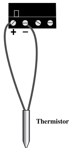
Wiring a Temperature Sensor
